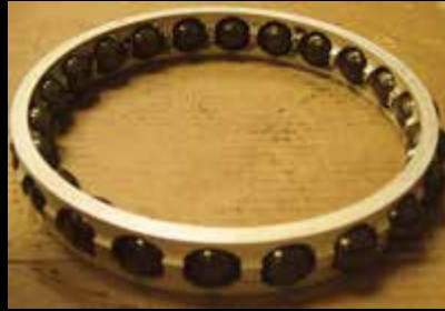
Mobil Jet Oil II in IAE V2500 No. 3 bearing Total engine hours: 35,937 Total cycles: 16,478
