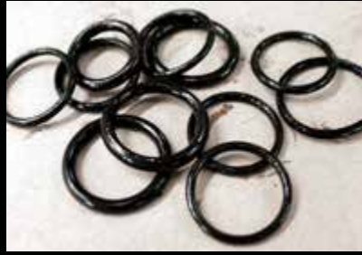
Mobil Jet Oil II in Honeywell TSCP 700 O-ring seals Since last repair: 2,891 hours; 2,638 cycles
