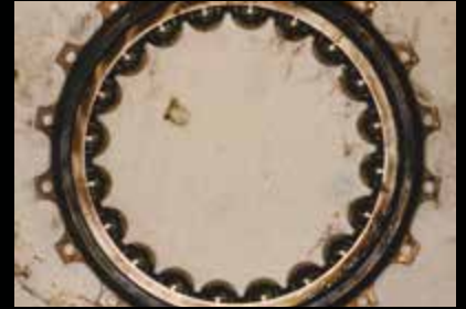
Competitive Type II oil in IAE V2500 No. 3 bearing Total engine hours: 13,588 Total cycles: 5,355
