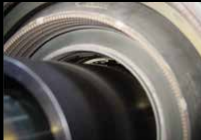
Mobil Jet Oil II in GE CF34 No. 5 carbon seal and bearing Total engine hours: 17,991 Total cycles: 14,988
